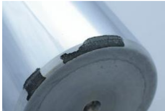
Figure 1. Piston with chipped coating; coating flakes can lead to contamination of food and beverage (BODYCOTE, 2017).
