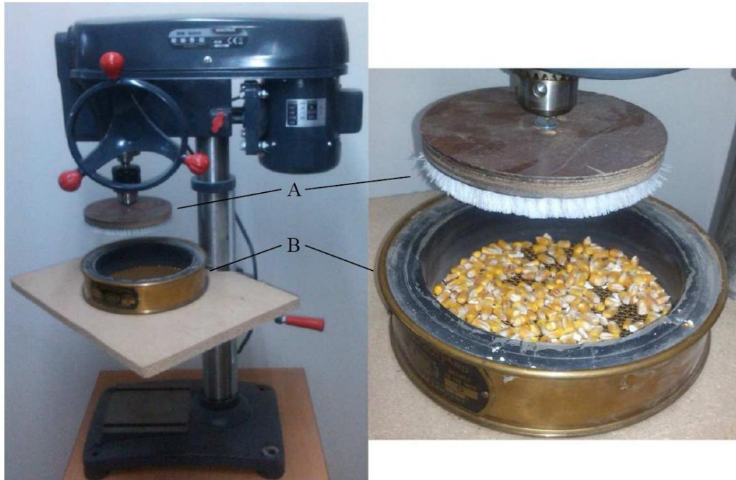
Figure 1. Laboratory grain brusher. A - fast rotating brush, B - motionless screen.
