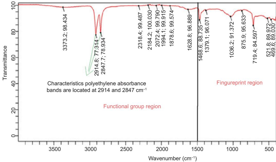
Figure 4. FTIR spectra confirming polyethylene (PE) type of microplastics.
