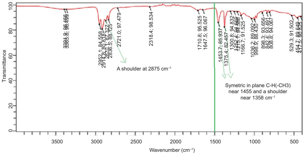
Figure 5. FTIR spectra confirming polypropylene (PP) type of microplastics.
